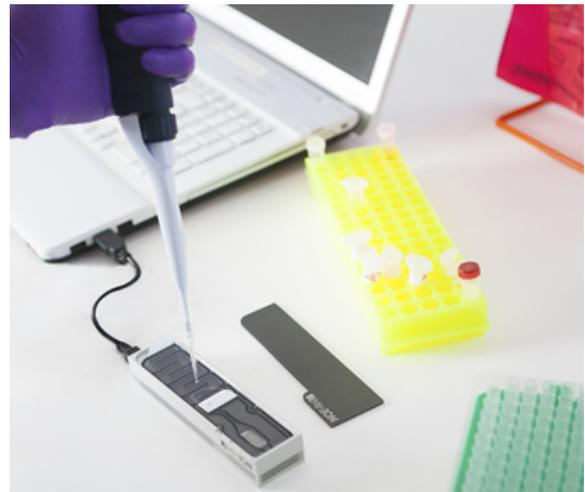
Fig. 1. An example of a miniaturised sequencing instrument.
