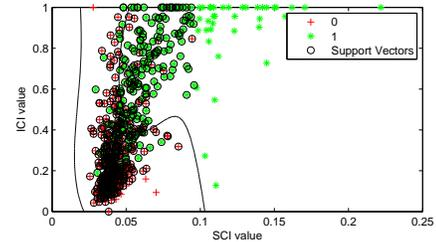
Fig. 3. Trained SVM classifier using SCI and ICI, where 1 indicates correctly identified vehicles and 0 indicates incorrectly identified vehicles
