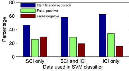
Fig. 4. Classification performance by using different kinds of data for the SVM classifier, such as SCI only, ICI only and the combination of SCI and ICI
