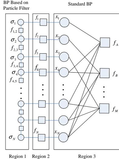
Fig. 1. Factor graph of belief propagation based on PF.
